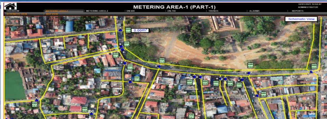
Map View of a Metering Area in SCADA
