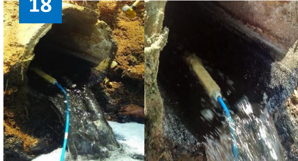
Municipal Corporation 1 - STP Sewage Inflow Survey: ❑ Identified 150% to 200% excess inflow than designed plant capacity.
