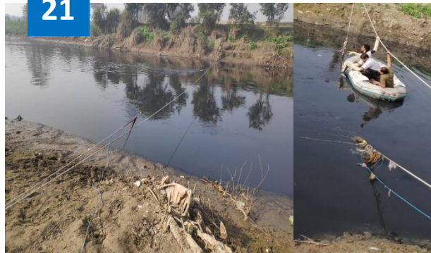
Flow Measurement Of Sewage Discharges Through Various Tributaries Into A Major River In North India.
